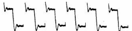
3. Square wave test on feedback amplifier showing peak at 9 times square wave frequency.
