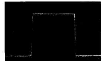
Fig. 2. Tracing of actual photograph showing 1.0 \mu sec pulse delivered by Model 212A.
