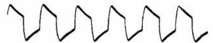
2. Square wave distortion from poor response at both high and low frequencies.
